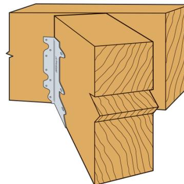
FIGURE 13B—TYPICAL SUR HANGER INSTALLATION
